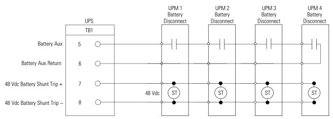
NOTE Battery aux and DC shunt trip wiring should be a minimum of 18 AWG.
